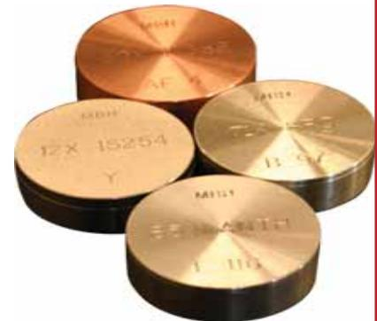
Typical XRF metal reference standards: thick, flat, smooth and homogenous.
