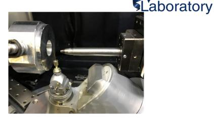
Pin diode mounted in front of the collimator
