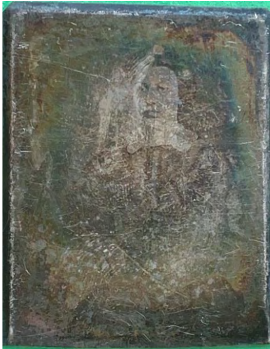
Optical image of a 1/9 plate daguerreotype photo that is mildly scratched and tarnished
