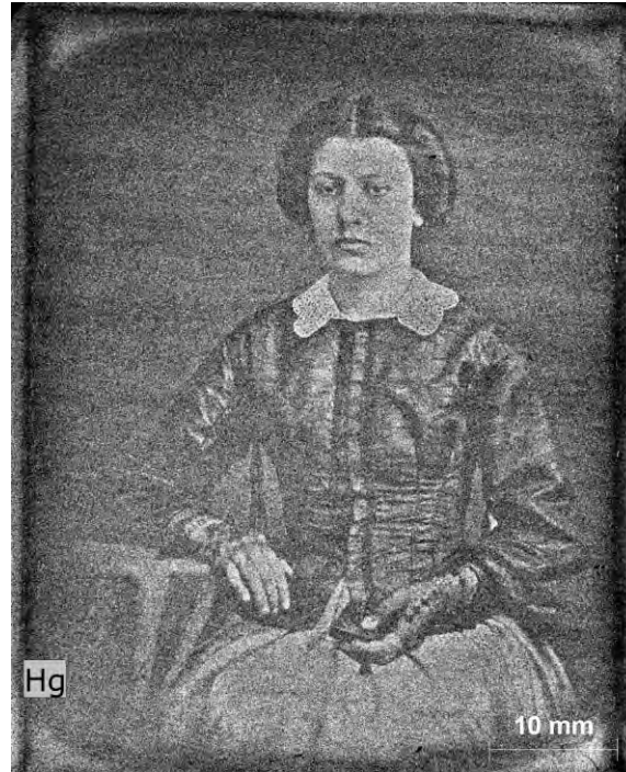
Hg image occurs as a "positive" due to the daguerreotype process, recovering fine detail
