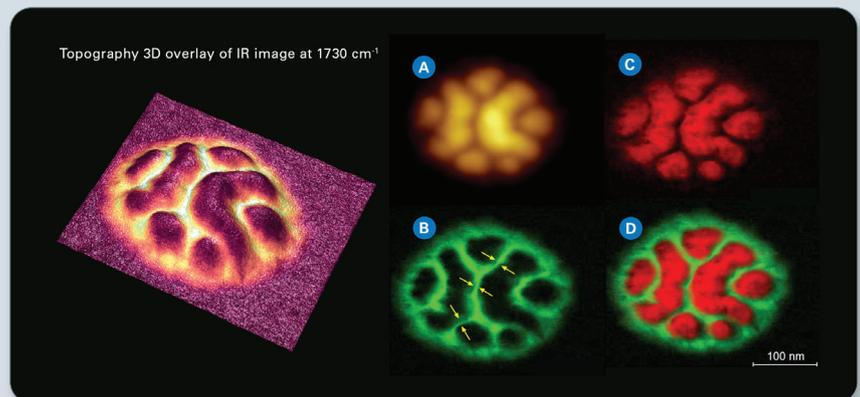
High-resolution chemical imaging of PS-b-PMMA block copolymer in Tapping AFM-IR mode showing sample topography (a); IR images at 1730 (b); and 1492 cm<sup>-1</sup> (c) highlighting PMMA and PS, respectively. The yellow arrows in panel (b) indicate chemical resolution <10 nm. The overlay image (d) captures the composition map.
