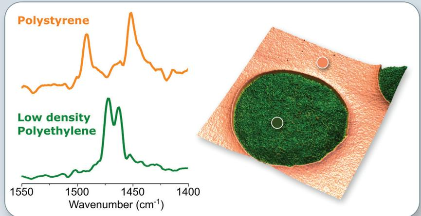
High-quality resonance-enhanced AFM-IR spectra collected at different sites on a PS-LDPE polymer blend, illustrating a high degree of material sensitivity and deeper insight into nanoscale material properties.
