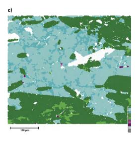
Likewise, silicate minerals often have very similar BSE intensities but phases such as Quartz, Albite and different Plagioclase minerals can be reliable differentiated with AMICS's advanced segmentation technology.
