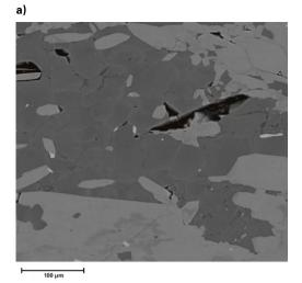
Figure 4 – Thin section of a silicate mineral BSE image (a), segmentation image (b) and resulting mineral maps after Particle mode (c) of a silicate containing thin section. A single frame was measured at 0.71 µm/pixel.
