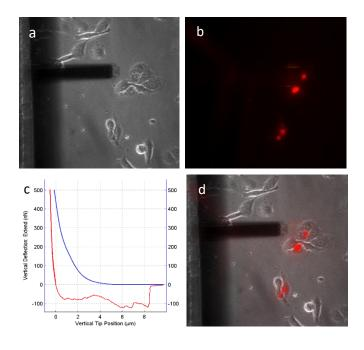
Fig. 6: Injection experiment (a) Phase contrast image (b) Fluorescence image after injection of propidium iodide (c) Force distance curve during injection (d) Overlay of phase and fluorescence image to demonstrate nucleus position
