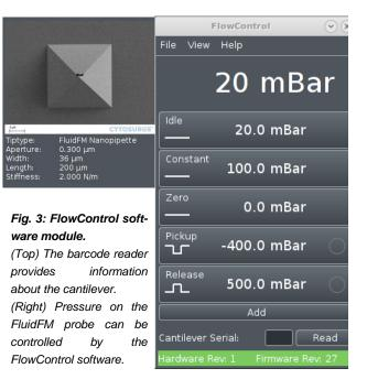
The FluidFM ADD-ON can be controlled from the same PC as the JPK BioAFM. The newly developed JPK FlowControl software module allows the user to define and set constant pressure or apply pressure pulses of defined lengths (Fig. 3). The intuitive handling of pressure control enables users to run complex experiments easily.
