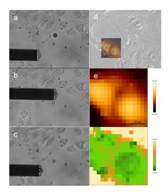
**Fig. 5:** Pick-up of a bead for Force Mapping on living cells. (a,b,c): Phase contrast images of living vero cells, the FluidFM micropipette and an 11  $\mu$ m polystyrene bead in front of it (a), during (b) and after pickup (c). (d) Overlay of optical image with Height map using the polystyrene bead. (e, f) Height and apparent stiffness map of two cells.
