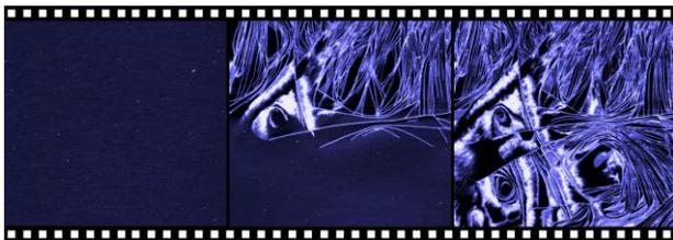
**Figure 5:** AM AFM phase images of a crystallizing PCL film at 61°C, 42°C and 42°C from left to right respectively. Scan range  $x = 4.2 \mu\text{m}$ ,  $y = 4.0 \mu\text{m}$ ,  $z\text{-range} = 13.5 \text{ degrees}$
