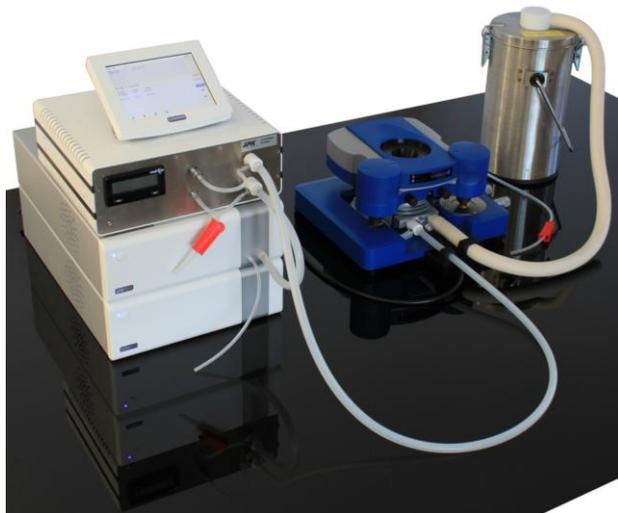
Fig. 1: JPK NanoWizard® on the new JPK CryoStage
