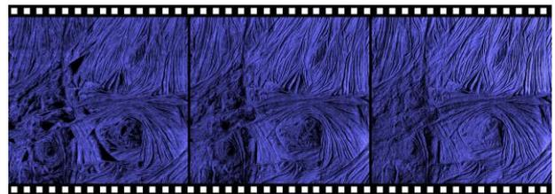
**Figure 6:** AM AFM phase images of a PCL film near and below glass transition temperature from left to right at -38°C, -55°C and -72°C, respectively. Scan range  $x = 4.2 \mu\text{m}$ ,  $y = 4.0 \mu\text{m}$ ,  $z\text{-range} = 13.5 \text{ degrees}$
