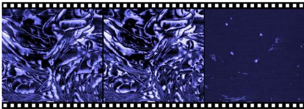
**Figure 4:** AM AFM phase images of a melting PCL film from left to right at 45°C, 65°C and 70°C, respectively. Scan range  $x = 4.2 \mu\text{m}$ ,  $y = 4.0 \mu\text{m}$ ,  $z\text{-range} = 13.5 \text{ degrees}$
