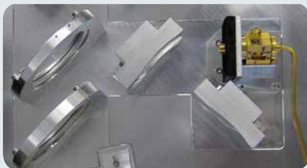
Quasi optical front-end of ELEXSYS-II E780
