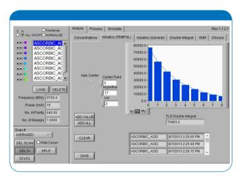
Double Integral values are calculated by the Processing and Analysis software, and plotted as a function of scan number. The time stamp on the data file is saved in the .csv output file.
