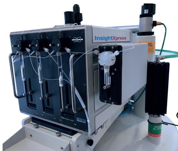
InsightXpress is a stopped-flow solution consisting of a pumping unit, a temperature controlled transfer line, a flow tube and software. The system is designed for seamless set-up in Bruker high-resolution NMR spectrometers with shielded magnets (300-700 MHz). Bruker's InsignMR™ software makes acquisition and analysis straightforward. It now has new functionality to enable the monitoring of very fast reactions.
