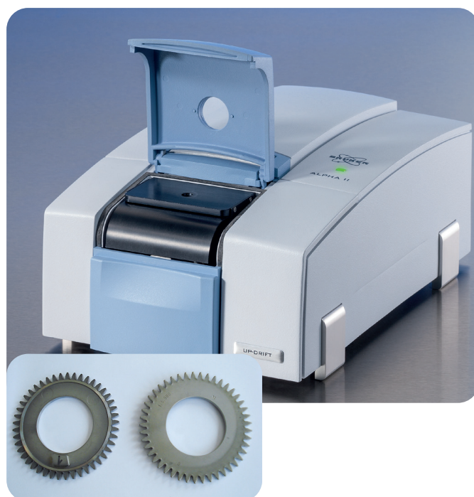
Figure 1: ALPHA spectrometer with the upward looking reflectance unit and the two different sides of a typical gear wheel (inset).
