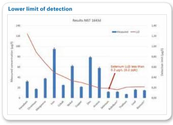
Water sample measurement of NIST 1643d standard by S4 T-STAR<sup>®</sup> and calculated LLDs show a detection limit for Se of < 0.2  $\mu$ g/L.
