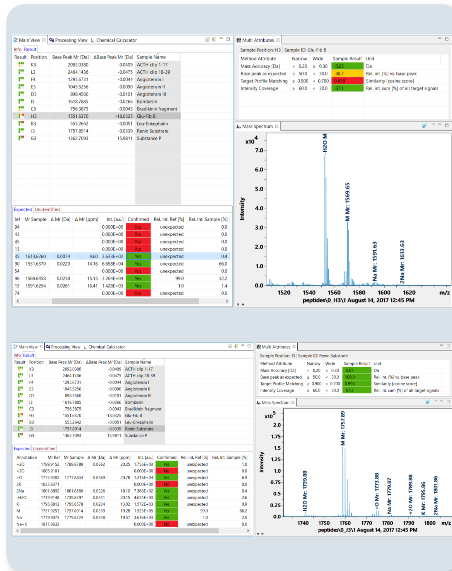
Fig. 3 Example MALDI analyses: Top Glu-Fib B represents a failed analysis requiring analyst inspection as the expected MH + peak has just 48.7% of the base peak intensity – due to loss of water (possible N-term pyro glutamylation). Bottom Renin substrate was automatically validated with 4 green quality attributes. All side products (water loss, oxidation and salt adducts) were only marginally detected.
