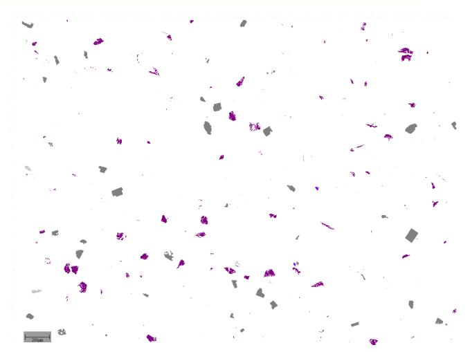
Measurement for only bright phases shortens measurement time to 14min
