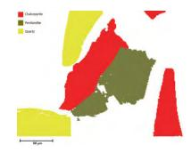
Resulting mineral map showing Chalcopyrite, Pentlandite and Quartz in Particle mode
