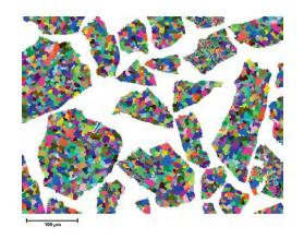
Particle segmentation image showing the result of segmentation of fine variations in BSE intensity
