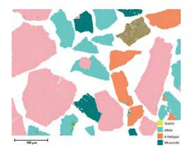
Resulting mineral map showing Quartz, Albite, Kfeldspar and Muscovite after Particle mode analysis Particle Segementation Example Differentate Chalcopyrite, Pentlandite and Quartz
