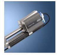
**SEM-EDS:** Analysis based on the sample interaction with an electron beam source from the SEM and the resultant X-rays that are detected using an EDS (simultaneous element detection)
