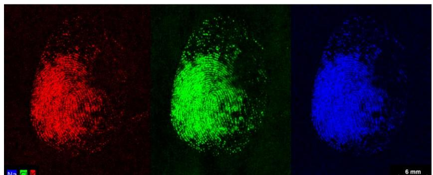
micro-XRF map of a fingerprint
