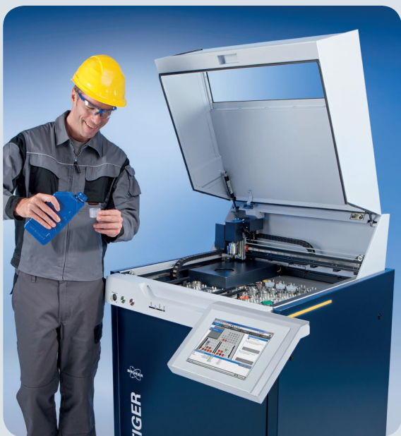
Figure 5: Easy and quick analysis of oil samples with PETRO-QUANT and the S8 TIGER
