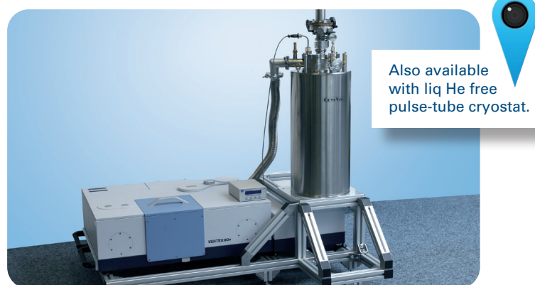
Fig. 8: Customized module for Silicon impurity photoluminescence, adapted to a VERTEX80v FTIR spectrometer. The samples are mounted in a liquid Helium bath cryostat in order to compensate the heat, created by the visible excitation laser
