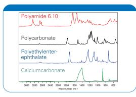
The IR-spectrum: Chemical fingerprint of polymers and auxiliaries.
