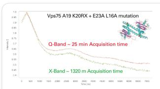
Acquiring the 4p-DEER spectrum at Q-band (red) results in a better signal to noise in only 2 % of the total acquisition time compared to acquisition at X-band (greed). Q-band data acquired with the QT-II resonator and 150 W TWT. X-band data acquired with MD-5 resonator and 1000 W TWT.
