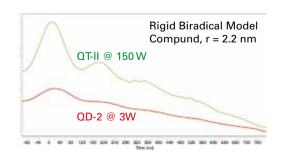
The QT-II with the larger sample volume and the Q-band TWT with more power provide a factor of 4 increase in the dipolar modulation depth (green) compared with the standard dielectric resonator and Q-band amplifier (red)
