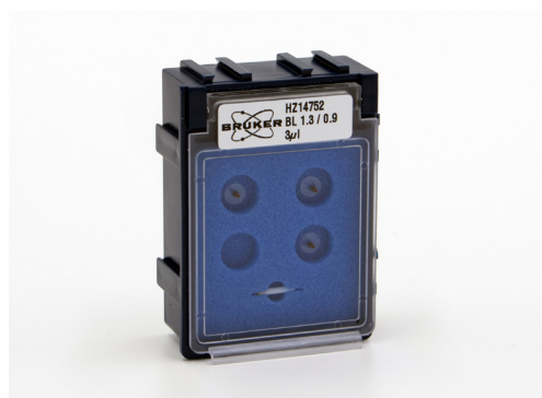
1.3 mm rotor kit ( HZ14752 )
