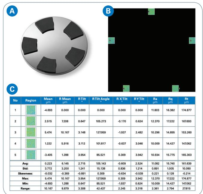
Figure 7. (a) Mounted Designed Pad structures, and (b and c) Automatic Analysis of Mounted Pad Conditioners.
