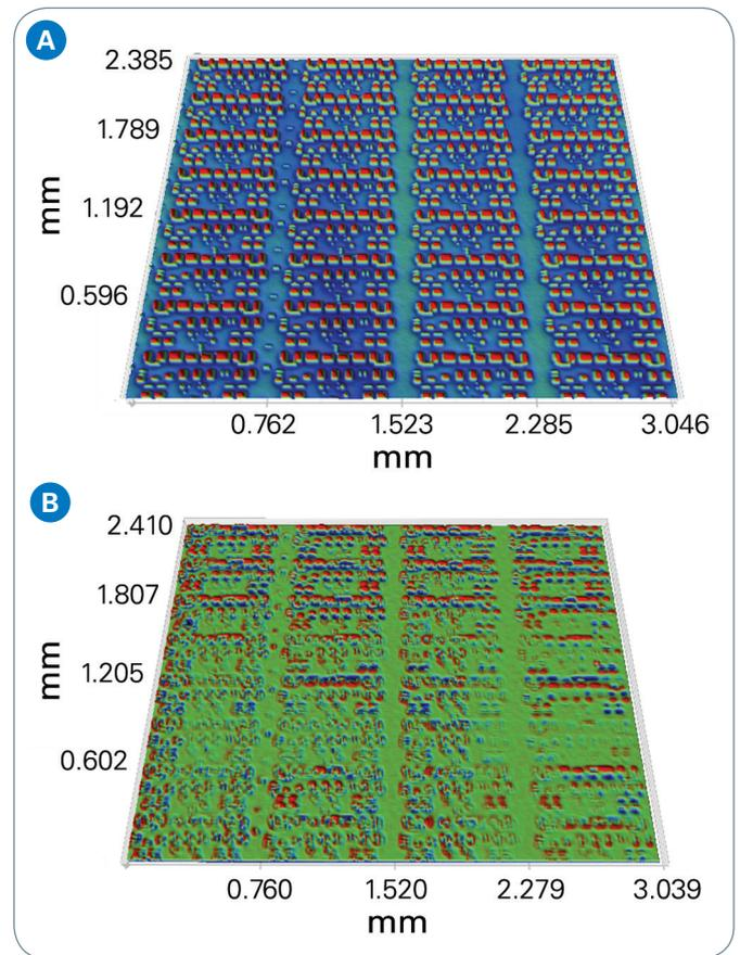
Figure 9. (a) Z-scaled  $\pm 70\text{nm}$  reference image, and (b) Z-scaled  $\pm 0.8\text{nm}$  subtracted image.
