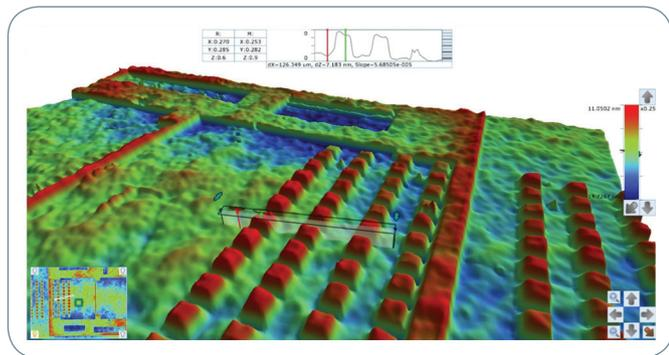
Figure 10. 4.6 x 2.5 mm field of view of a CMP-processed wafer with nanometer structures and T-Box openings.
