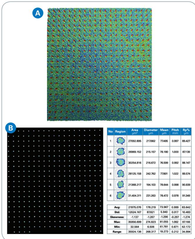
Figure 4. (a) 3D optical image of designed pad, and (b) automatic detection/analysis of the designed pad conditioner.
