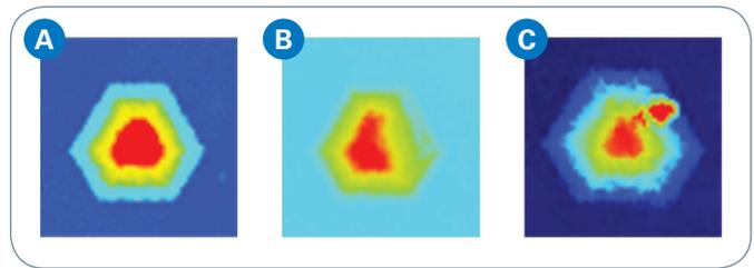
Figure 6. (a) Good structure, (b) missing peak causing LOW Rp%, and (c) debris causing HIGH Rp%.
