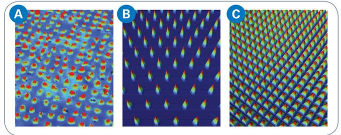
Figure 3. (a) Diamond pad versus two DLC-coated designed-structure pad conditioners (b and c).
