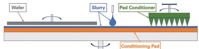
Figure 1. Typical functional principles of a CMP process.
