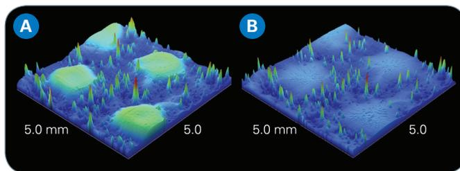
Figure 11. (a) Diamond before testing, and (b) the same diamond after the wear test.
