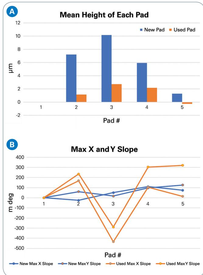
Figure 8. (a) Pad mean height versus (b) X–Y pad tilt angle of a new, good pad versus a used, bad pad.
