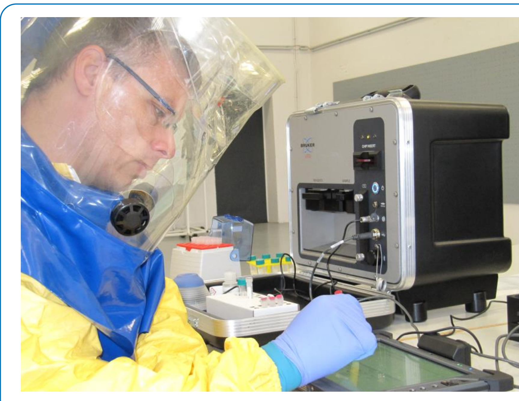
Fig. 2 End user test in course of GEFREASE project. pBDi operated with personal protective equipment by French and German fire fighters.
