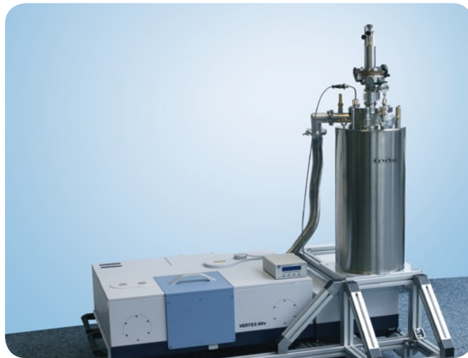
Fig. 8: Customized module for Silicon impurity photoluminescence, adapted to a VERTEX 80v FT-IR spectrometer. The samples are mounted in a liquid Helium bath cryostat in order to compensate the heat, created by the visible excitation laser
