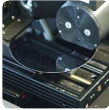
Automated x,y stage for laterally resolved photoluminescence mapping.
