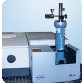
Cryostat adaption for low temperature photoluminescence spectroscopy.
