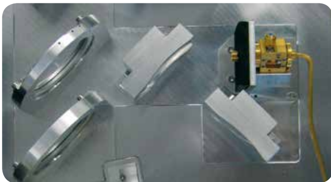
Quasi optical front-end of ELEXSYS E780
