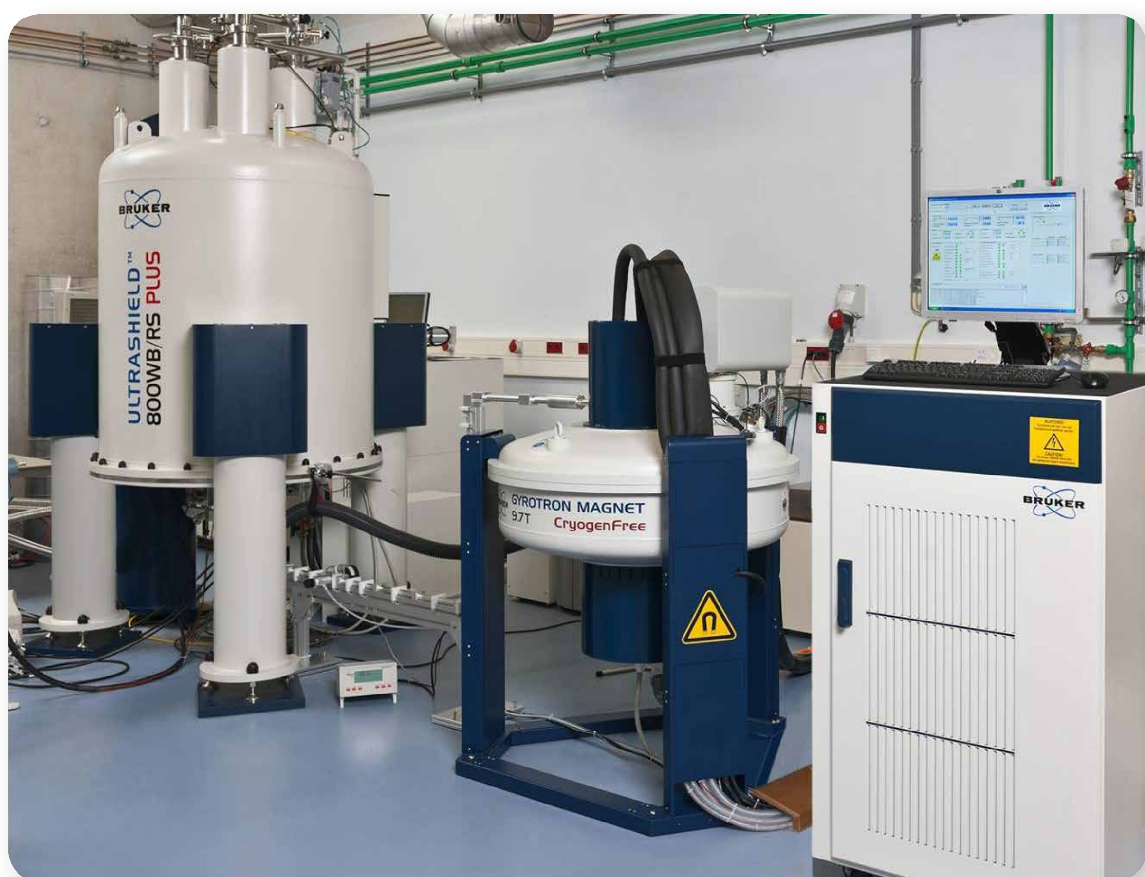
Fig. 1 Photograph of 527 GHz DNP Spectrometer at the University of Utrecht, The Netherlands. Left to right: 800 WB NMR magnet, microwave transmission line, second-harmonic cryogen-free gyrotron tube and magnet, control system.
