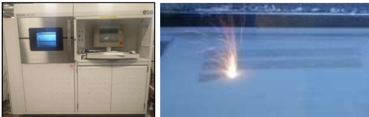
Figure 1: An EOS M270 SLM system used for specimen fabrications (left) and a photo showing SLM process (right).
