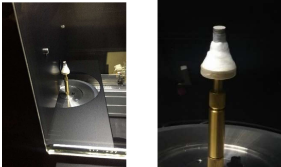
Figure 3: Specimen setup in the CT system showing near x-ray window (Left) and closed-up view (Right).
