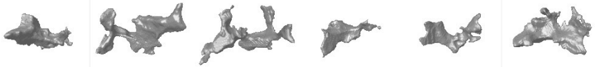
Figure 5: 3d models of some of the largest particles of the sulfide phase.
