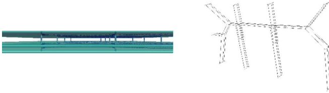
Figure 9. An artificial “sandwich” image (three horizontal plates connected by orthogonal rods, light blue on the left) leads to the creation of artefactual 3-connected “trabecular” junctions with maximal spanning angles.
