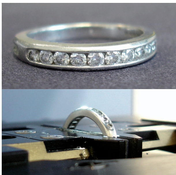
Figure 2: Diamond ring fixed in the sample holder vice on the LUMOS stage.
