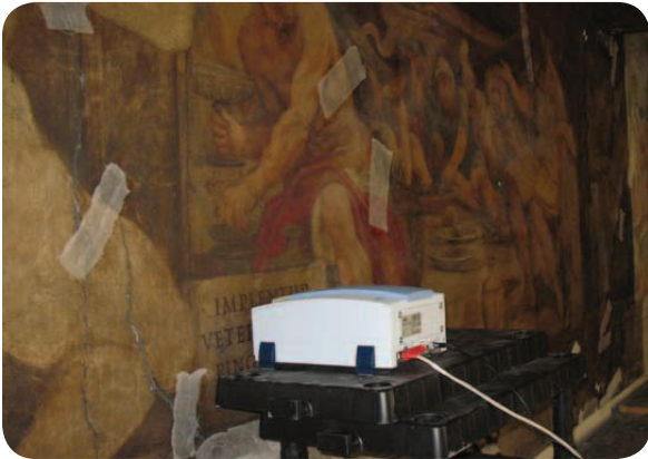
Figure 2: The ALPHA, equipped with a dedicated reflection module, is placed in front of the mural painting to perform the FT-IR measurements.
