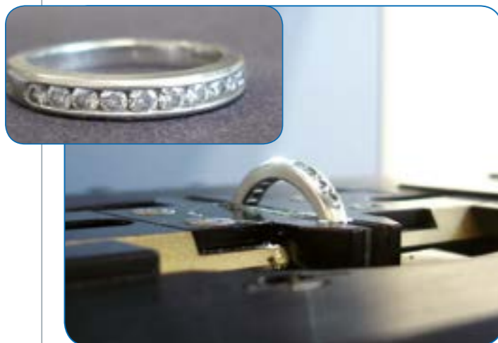
Figure 9: Diamond ring fixed in the sample holder vice on the LUMOS stage.
