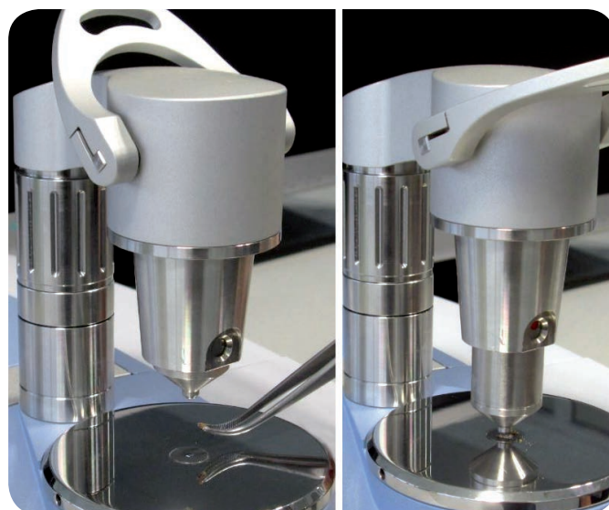
Figure 1: A kidney stone sample is being pressed on the diamond ATR crystal.
