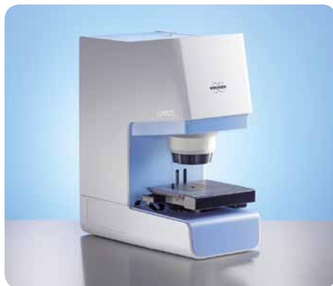
Figure 1: Stand-alone FT-IR microscope LUMOS.
