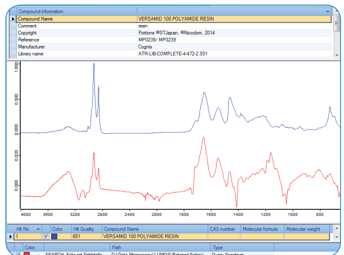
Fig.3 a: Identification of the additional component in the spectrum of the defect (red) by search of the difference spectrum between the query spectrum and the library spectrum of the basic foil material.
