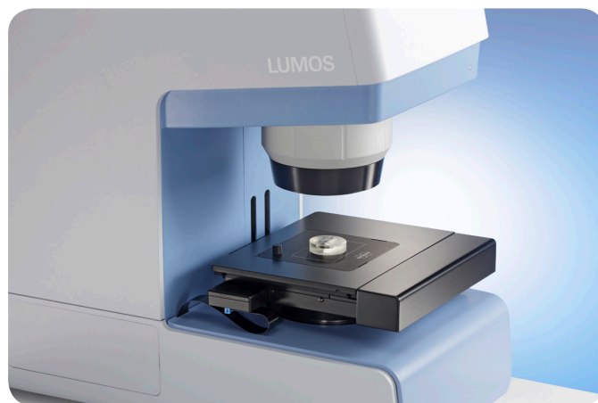
Fig. 3 Sample on the stage of the LUMOS FT-IR microscope
