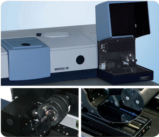
Fig. 1: Top: PII module adapted to VERTEX 70 research FT-IR spectrometer. Lower left hand side: standard glass objective with vertical sample mount. Lower right hand side: mirror objective and X-Y mapping stage for convenient horizontal sample positioning.
