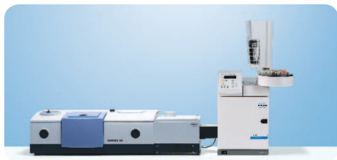
Picture 1 GC-IR accessory placed in between the GC and the FT-IR
