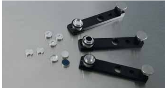
Figure 8: The picture shows the supplied three different sample mounts together with the available sample cups
