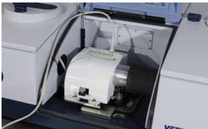
Figure 3: Detailed look at the PAS cell mounted inside the spectrometer sample compartment showing the inserted sample carrier.
