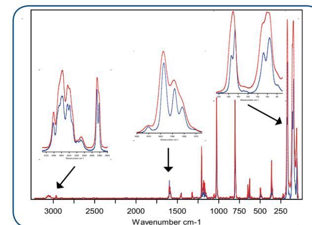
SENTERRA II provides the full spectral range even at high resolution. Spectra of triptycene measured at a resolution of  $4 \text{ cm}^{-1}$  (red) and  $1.5 \text{ cm}^{-1}$  (blue).
