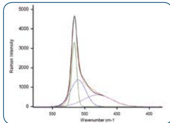
Characterization of the crystallinity of a silicon thin film on a solar cell. The spectrum (red) was measured with very low power to avoid any sample damage.
