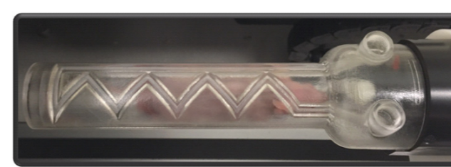
Figure 2: FML lid installed on MMAB base and mounted to Albira MMAB docking arm.
