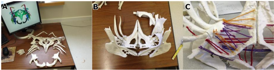
Figure 4: Rapid prototyping. By using a rapid prototyping machine, we generated a twenty times up-scaled physical model of the clingfish suction disk. A: The bones of the suction disk were created as individual elements based on the segmented micro-CT data. B: The individual pieces were then reassembled. C: Yarn was used to highlight the position of muscles in the clingfish suction disk.
