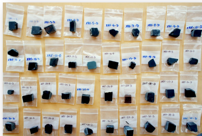
Figure 3. Photograph of the 40 obsidian calibration samples. Each ziplock bag is 5 x 8.5 cm.
