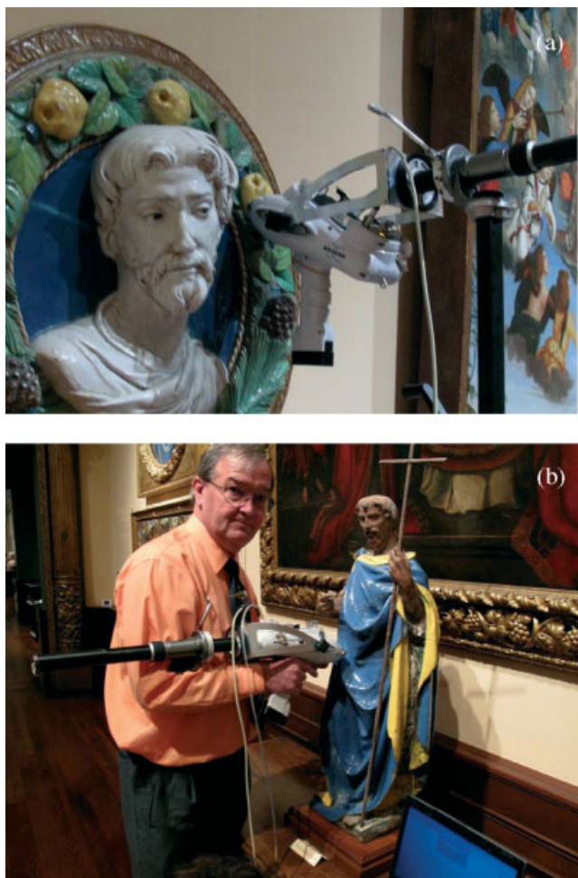
Figure 1. On-site handheld EDXRF data collection Saint John the Baptist (tondo) (a) and Saint John the Baptist with Cross statue (b).
