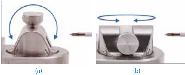
Fig. 2 Schematic representation of a) the tilt stage and b) the rotation stage, available accessories for the Hysitron PI 88 SEM PicoIndenter.
