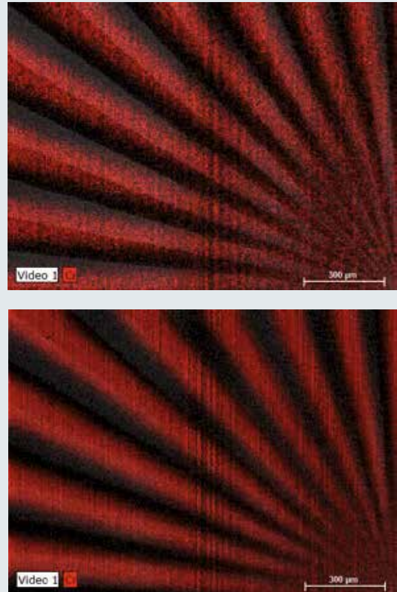
Fig. 4 Images of a Siemens star for same spot size but different acquisition time per pixel: 5 µm/5 ms (top) and 5 µm/50 ms (bottom)
