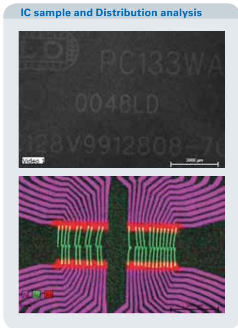
Fig. 7 Image of an IC and the elemental distribution of Ni, Ag and Au that shows the lead frame together with Au-bonding
